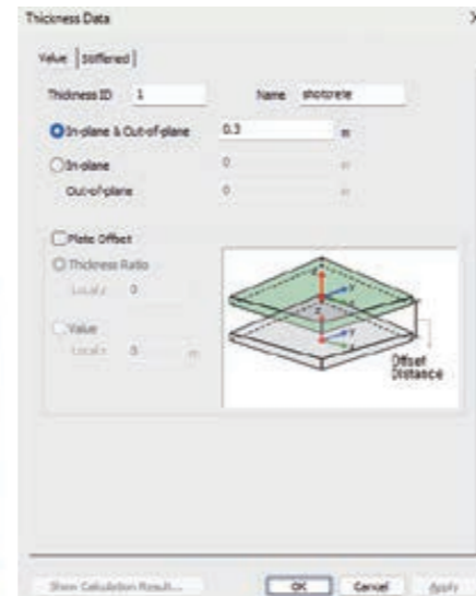
3. SKELETON WITH SHOTCRETE (thickness of shotcrete)
