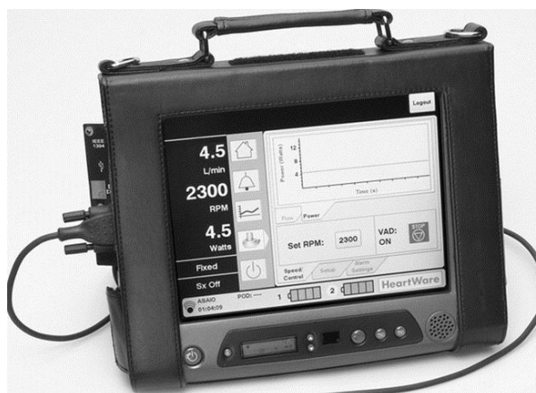
Figure 1.11 – Monitor display of the HVAD 29 .
