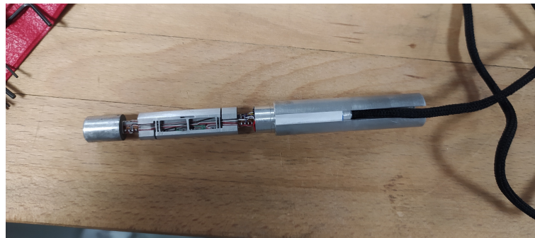
(a) Sting balance without the metal cover.
