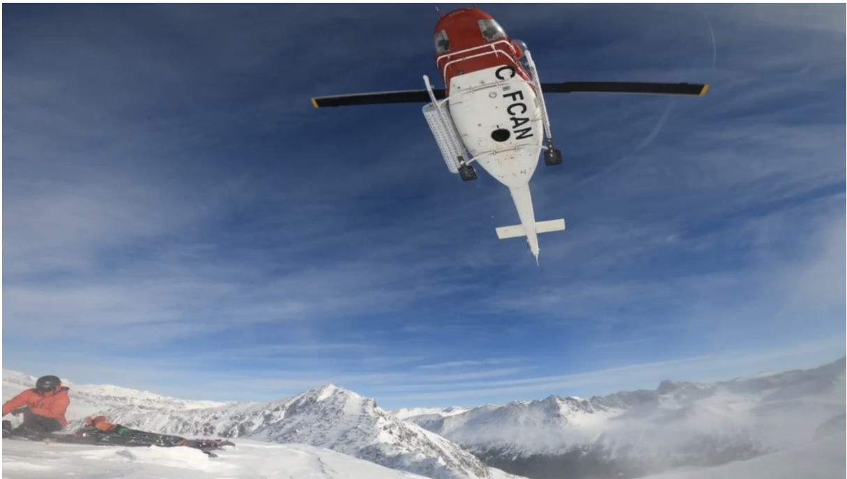
Figure 1: Bell 212 helicopter taking off in mountainous conditions. Powder snow lifted from the ground makes wingtip vortexes visible - Personal shot
