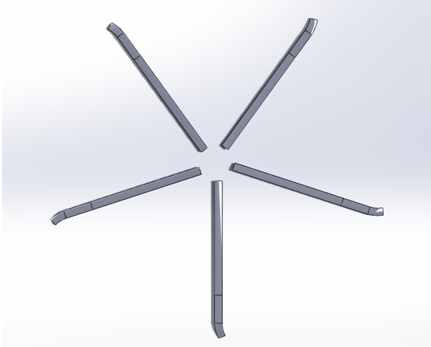
Figure 3.6: Rotor view from the top. Tip sweep is clearly visible
