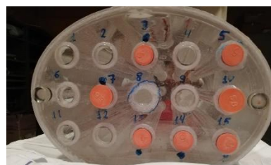
Figure 3: View of the cannels in the phantom (channels contain detectors + polyethylene spacers).
