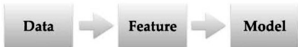
Figure 1.9: The pipeline of building a machine learning system, consisting of three major steps of data collection, feature generation, and model training[36]
