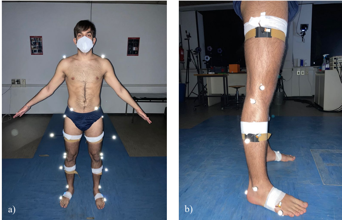
Figure 18. Positioning of makers and IMU sensors, (a) frontal and (b) lateral view.
