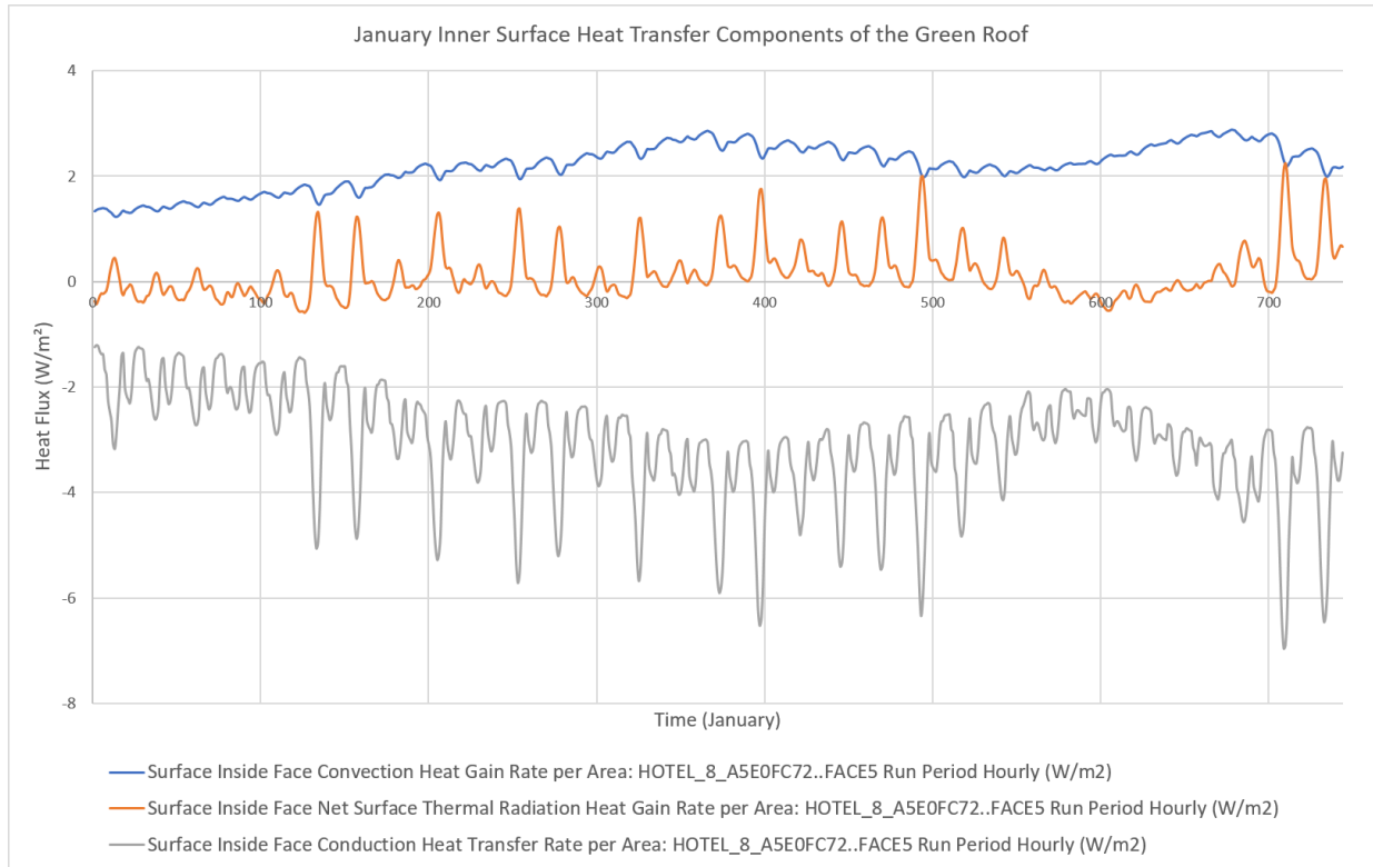
Figure 37, Hourly variation of convection, net thermal radiation, and conduction heat transfer rates at the inner roof surface under green roof conditions during January
