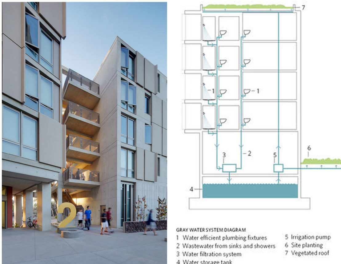
Figure 46: Water recycle system Source: AIA Top Ten. 2013
