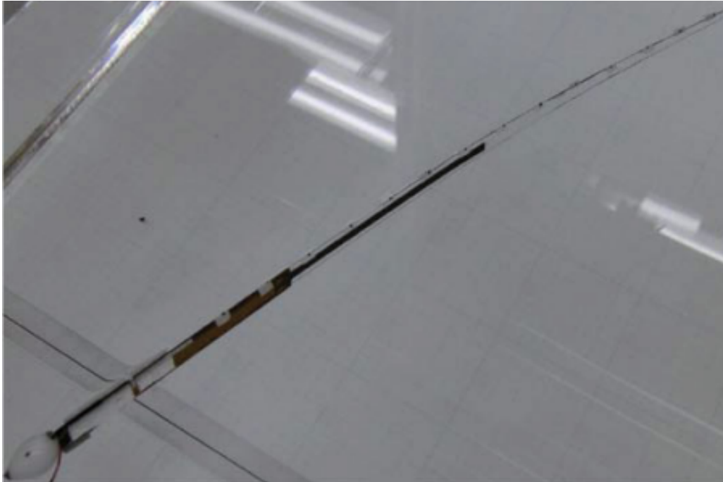
Figure 2.1: Prototype of snake robot built using piezoelectric fiber composite [46]
