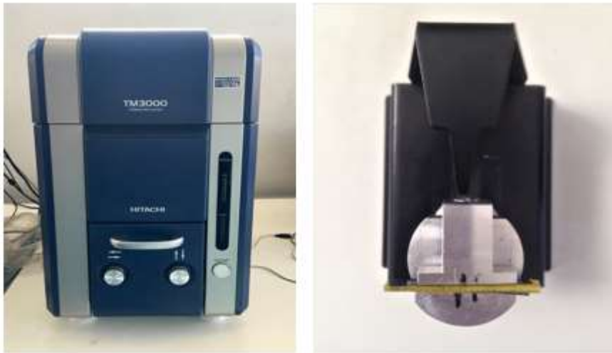
Figure 23: Hitachi TableTop SEM (on the left) and a top view of the SEM holder blocking the composite specimen covered with conductive tape.
