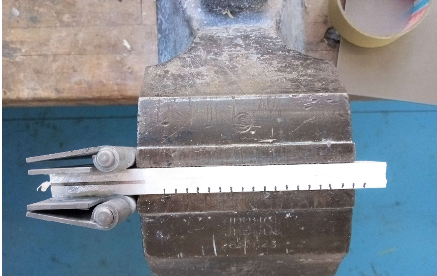
Figure 52: Assembled DCB specimen secured in the vice.
