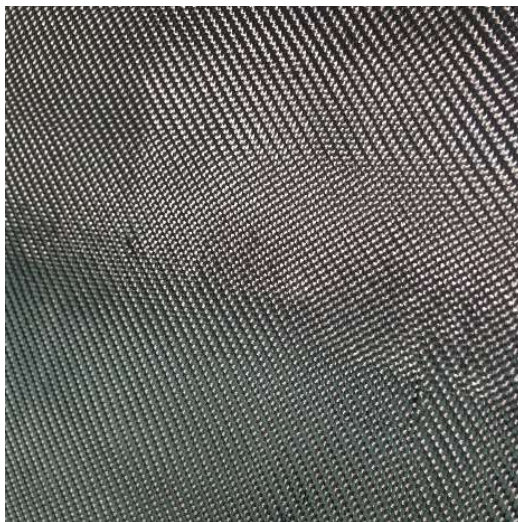
Figure 35: Zoomed photo of the E-glass woven fabric used to design the composite panel.
