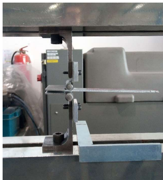
Figure 53: Preliminary DCB test to verify the surface treatments adopted for the second panel.
