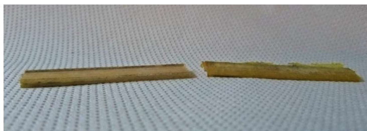
Figure 43: Comparison between a non-lapped specimen (left) with a lapped one (right).
