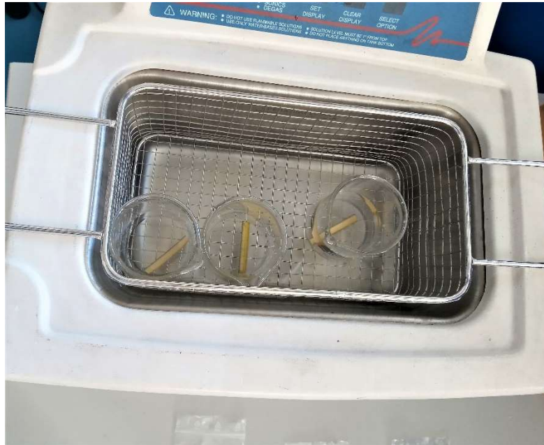
Figure 44: SEM specimens (P1, P2, P3) plunged in ultrasonic bath.
