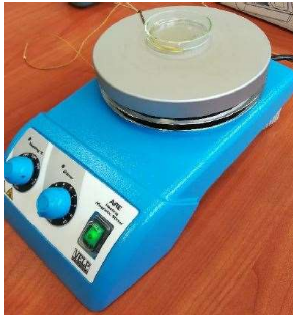
Figure 34: VELP Scientifica ARE magnetic stirrer supplied by DAER laboratory for resin preparation.
