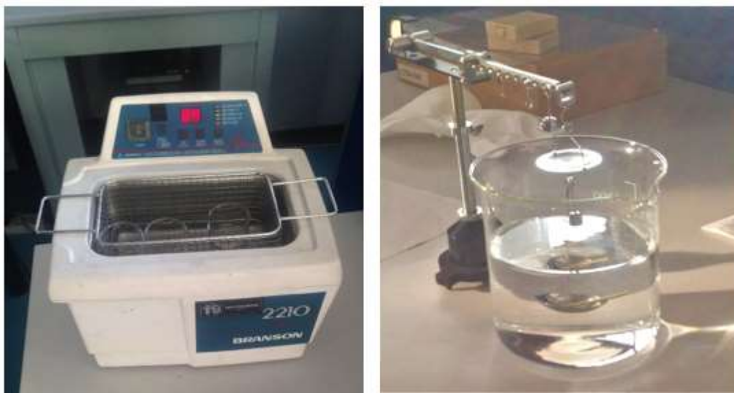
Figura 24: Westphal balance (on the right) and Branson ultrasound bath (on the left) at the disposal of DAER laboratory.
