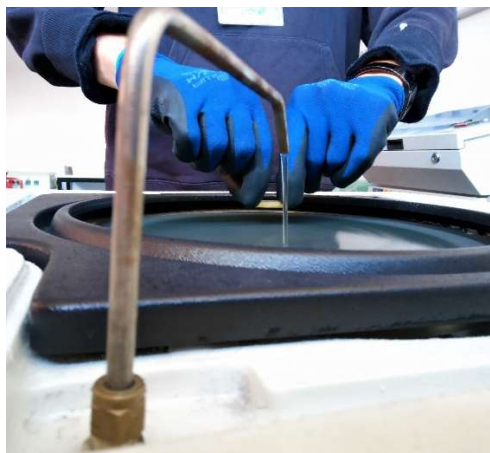
Figure 42: Lapping of SEM specimens.
