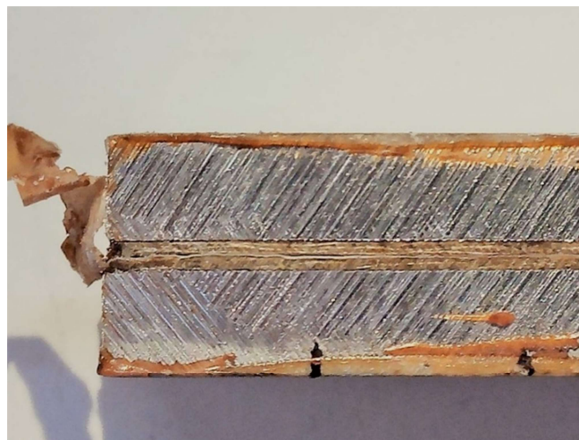
Figure 70: Mid-plane zoomed image of the repairing effect.
