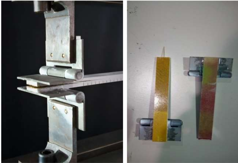
Figure 66: Evidence of the interface collapse during (on the left) and after (on the right) the DCB test.
