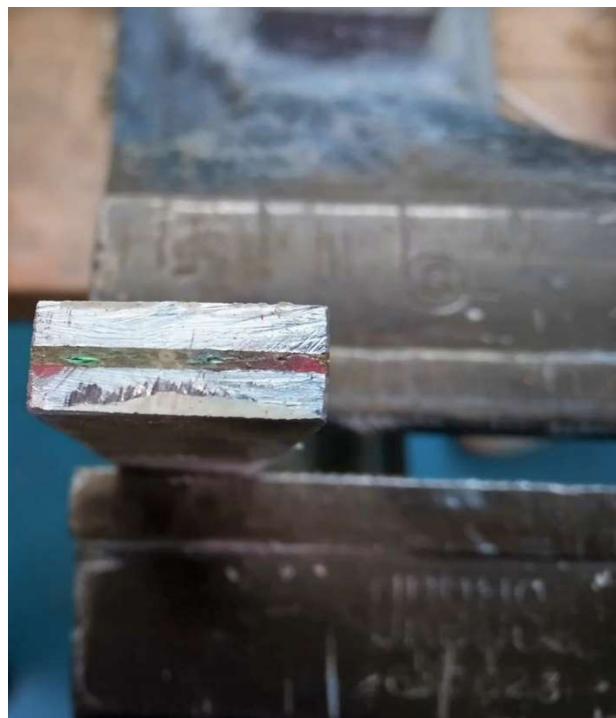
Figure 33: Proof of the mechanochromic effect (green spots) caused by accidental scratches during manufacturing.
