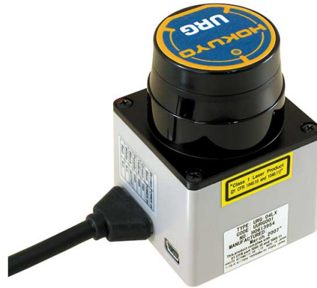
Figure 4.4: Hokuyo URG-04LX-UG01 laser sensor mounted on the reference robot
