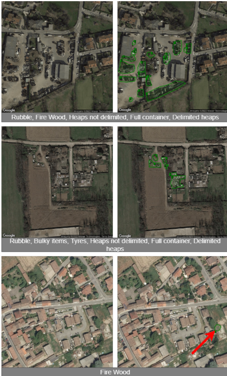
Figure 3.5: Examples of testing images from the AerialWaste data set [18]. On the right, segmentation masks are shown. As it is possible to see, annotating the data set can be very complicated given that many objects are present in the same image, and sometimes, the objects of interest cover a minor portion of the image.
