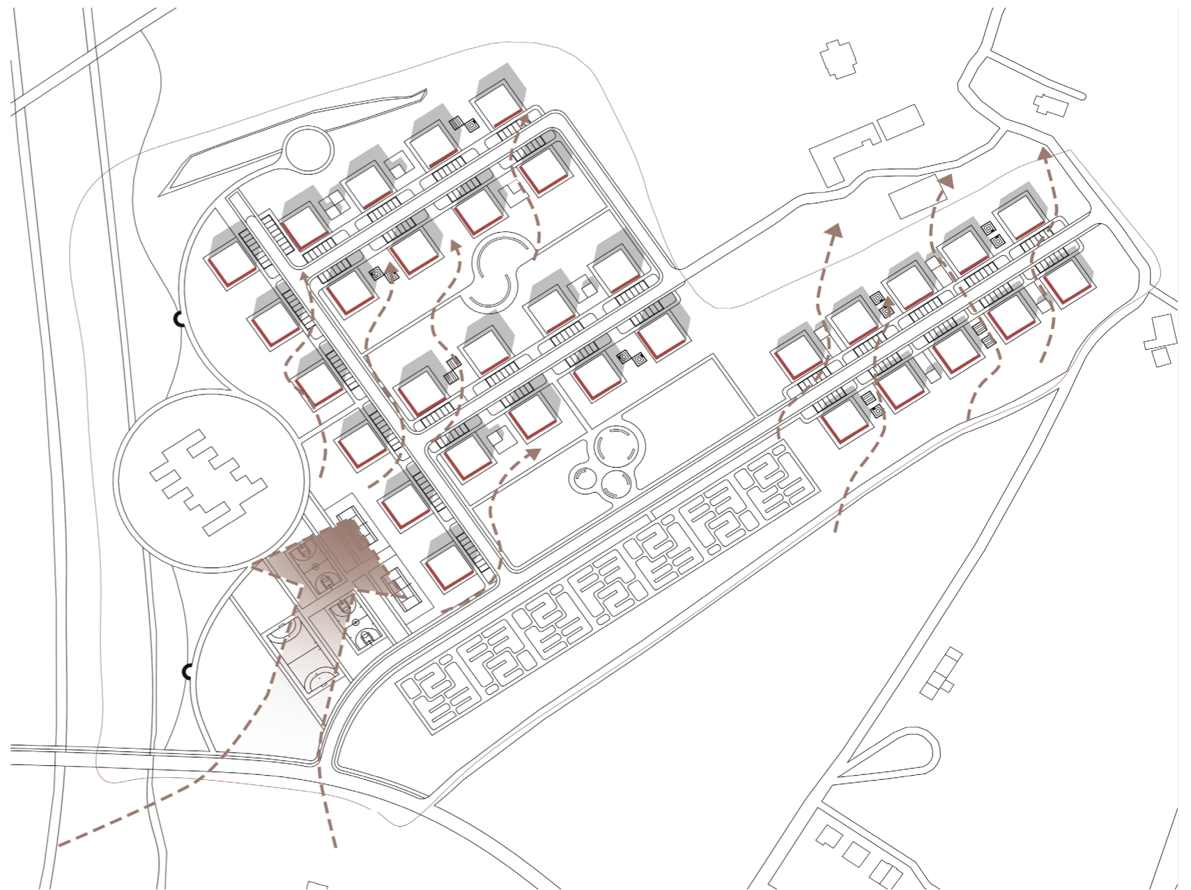
Fig.42. Diagram showing the logic of units placement according to wind;
