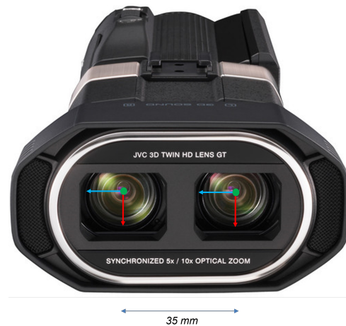
Figure 3.2: Vision sensor: JVC GS-TD1 Full HD 3D Camcorder.
