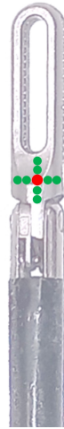
Figure 3.16: The 9 points tracked by the Optical flow (in red the point found by the CNN, in green the surrounding points).
