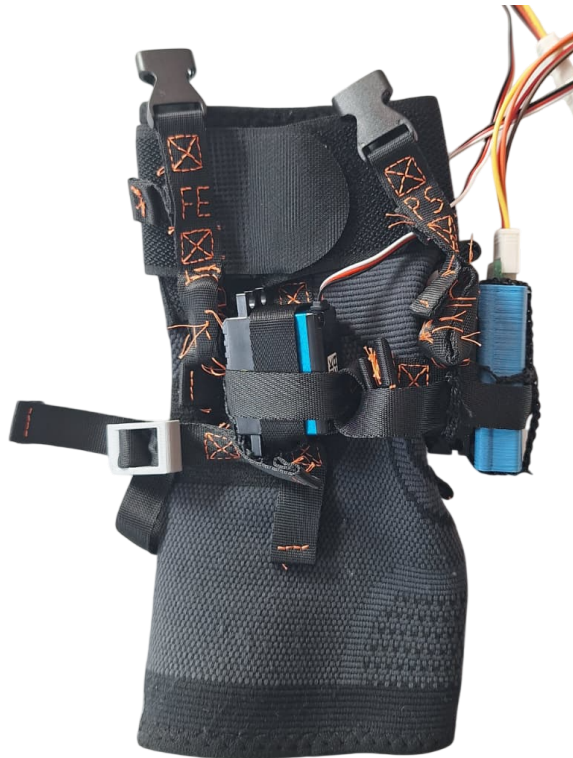
Figure 2.47: Forearm sleeve with one servo motor on the top and one servo motor and one IMU on the right, corresponding to the elbow side.
