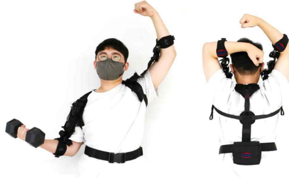
Figure 1.18: Soft exosuit for elbow flexion/extension actuated by fabric SMA muscle from [51].
