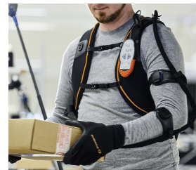
Figure 1.34: Ironhand - commercial soft exosuit for fingers flexion for industrial applications with cable driven actuation from [8].
