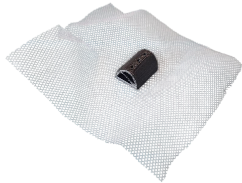
Figure 2.39: Palmar protrusion 3D printed directly onto a porous gauze fabric base to allow for textile integration.
