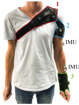
Figure 1.31: Soft exosuit for elbow flexion/extension with tendon driven actuation from [42].
