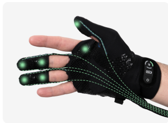
Figure 1.33: Carbonhand - commercial soft exosuit for fingers flexion for health-care assistance and rehabilitation with cable driven actuation from [8].
