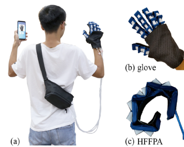
Figure 1.16: Soft exosuit for fingers flexion/extension with pneumatic actuators equipped with strain limiting layers from [20].
