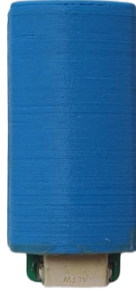
Figure 2.31: 3D printed casing containing the IMU BNO055 from Bosch.
