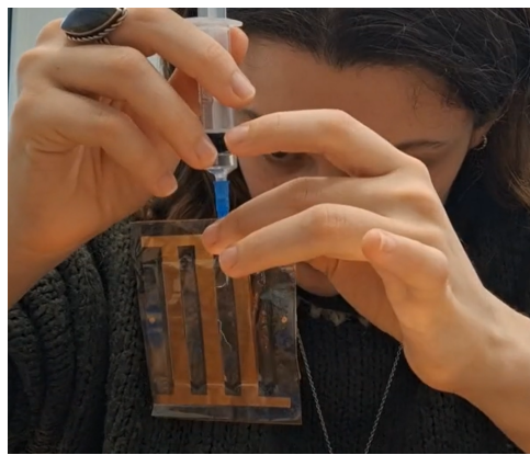
Figure 1.39: HALVE actuator being filled with oil using a syringe with a filed tip not to break the Mylar ® film.
