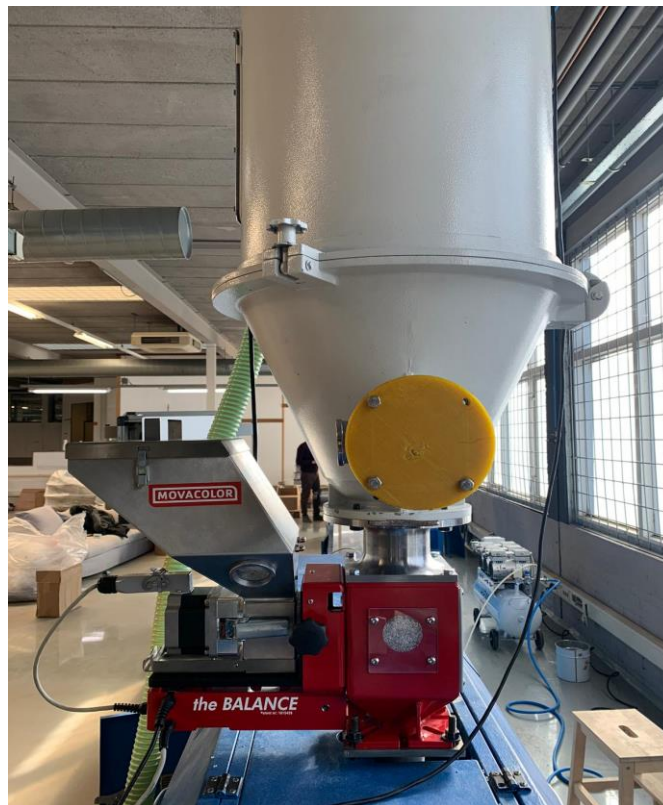
Figure 21 - Colour Mixing Equipment
