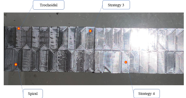
Figure 1: Two machined aluminium billets. The four different adopted machining strategies can be noted on the surface. Each machined rectangle represents a sample.
