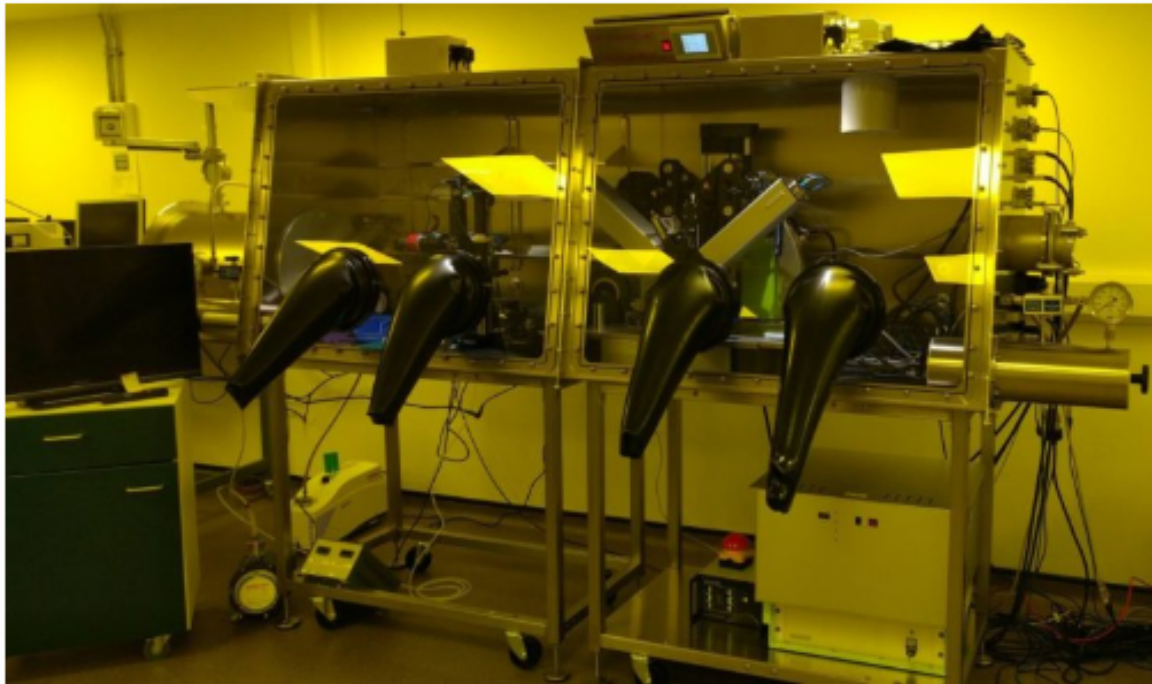
Figure 5.3: Clean room facility of the department of Physics at Heriot Watt University (UK). In this photo is displayed the glovebox used during the first part of this experimental thesis. It is equipped for 2D fabrication and ellipsometric characterization of thin films in an inert environment.
