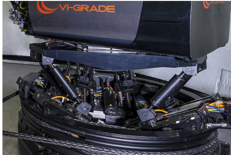
Figure 1.7: Hexapod under the cockpit of the simulator[12]
