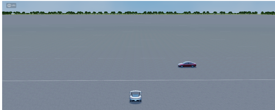
Figure 2.2: This is the first test when the car at 25m passes in front of the driver
