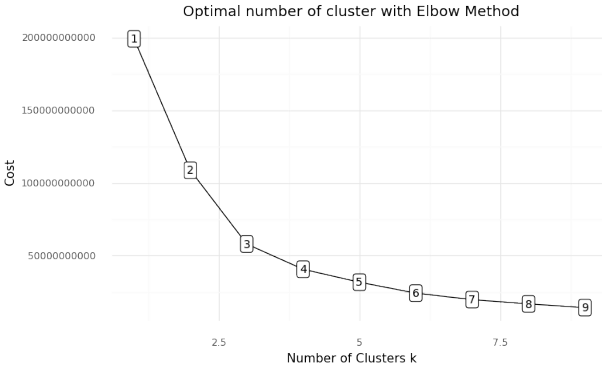
Figure 4.1: Cost of the clusterization task from 1 to 9 clusters using the Elbow Method.
