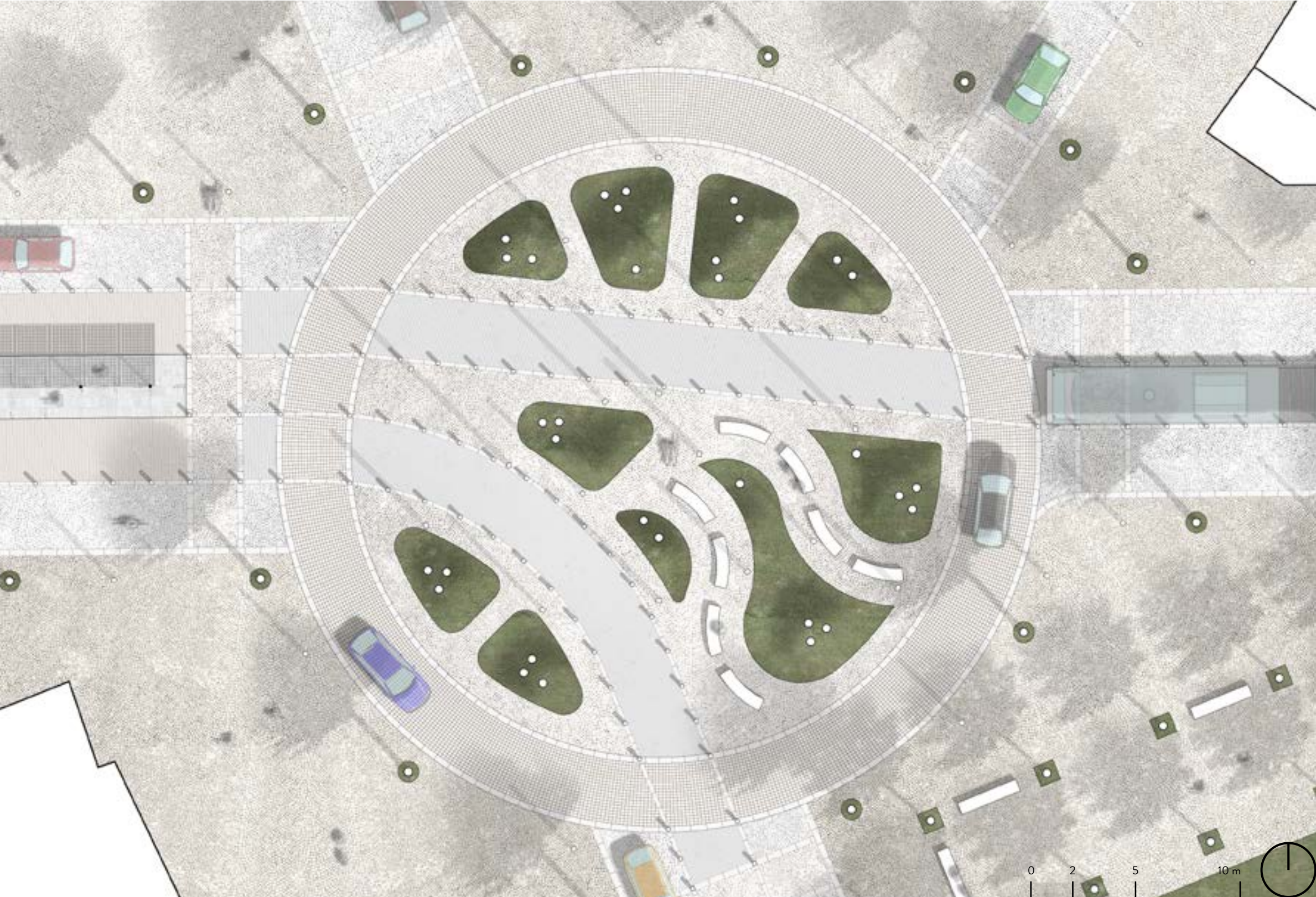
Fig. 60 - Design solution: Roundabout
