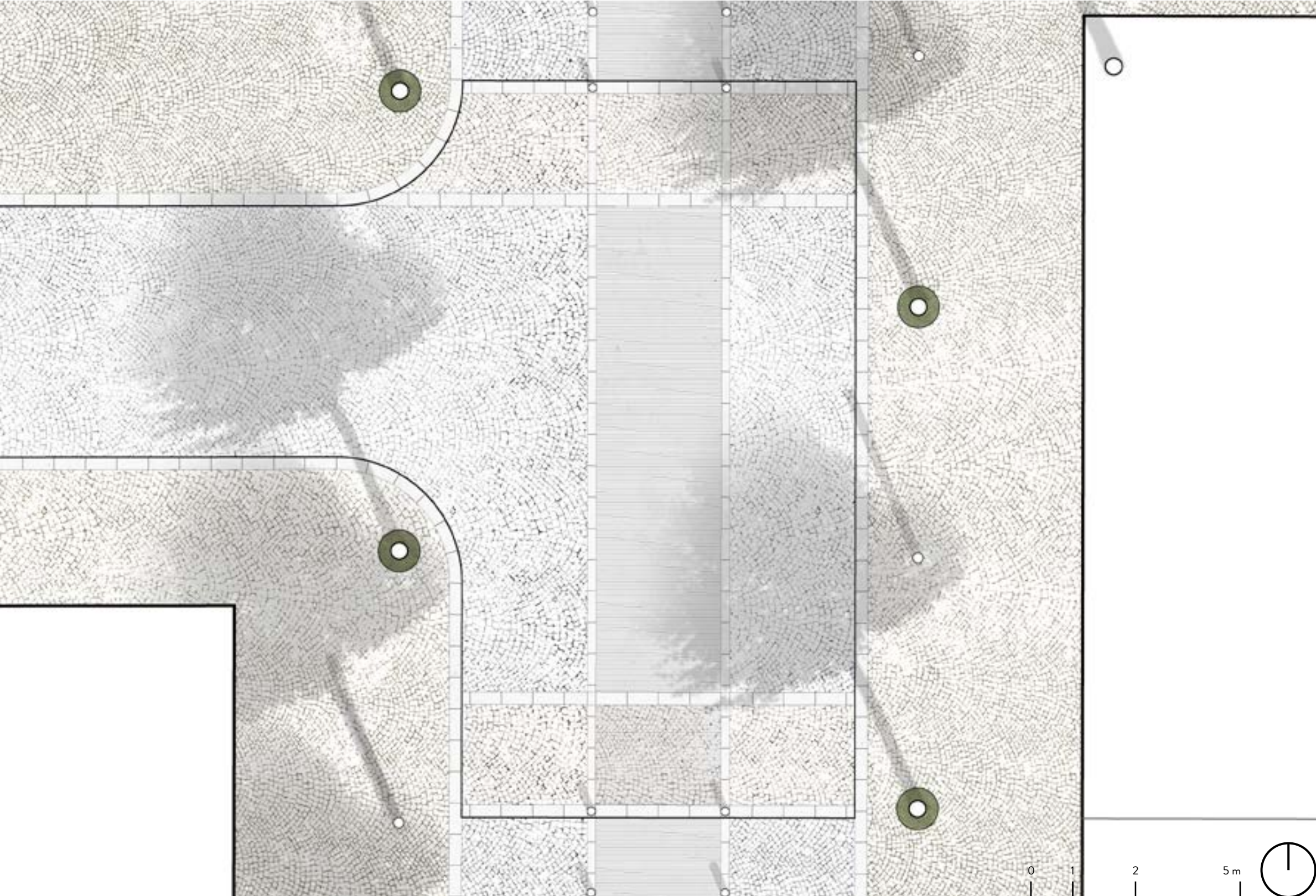
Fig. 63 - Design solution: Pedestrian crossing at shared level
