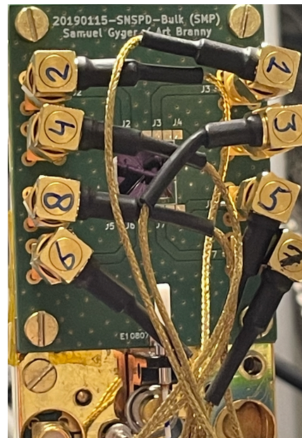
Figure 7.2: open PCB in cryostat with fiber end
