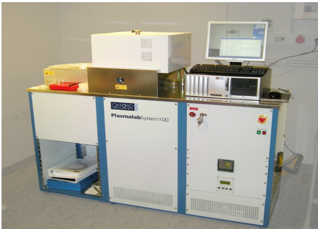
Figure 3.6: Oxford Plasmalab 100 for RIE etching
