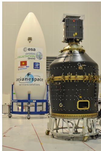
Figure 4.1: Proba-V mounted on VESPA, from [1]
