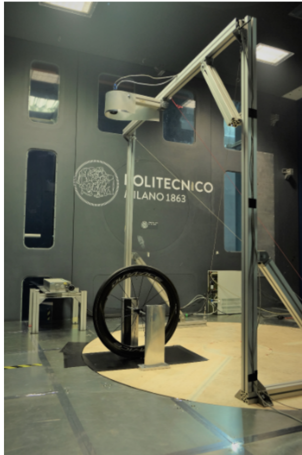
Figure 4.1: Detail of wheel support NACA 0021 profiles and PIV setup.
