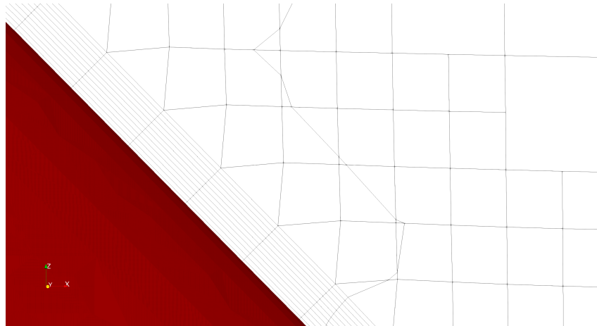
Figure 3.7: Layers on the rim and spokes after the snappyHexMesh layer addition phase meshing process.
