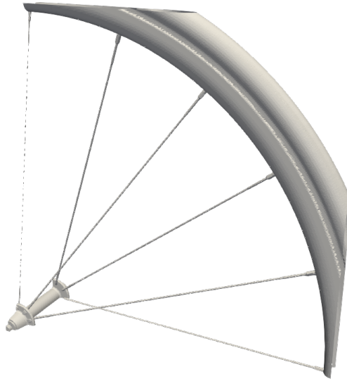
Figure 3.6: Surface details of the rim and spokes after the snappyHexMesh meshing process.
