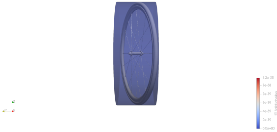
Figure 3.15: MRF configuration 1, r = 34\text{cm} , front view, case yaw angle = 20^\circ
