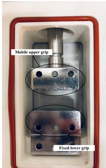
Figure 29 Test chamber containing the clamp instrument. The upper grip is the mobile one while the lower is fixed
