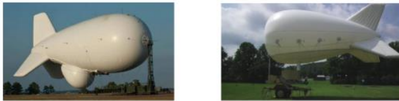
Figure 15: airborne aerial platforms, a. JLENS program, b. REAP aerostat [3]
