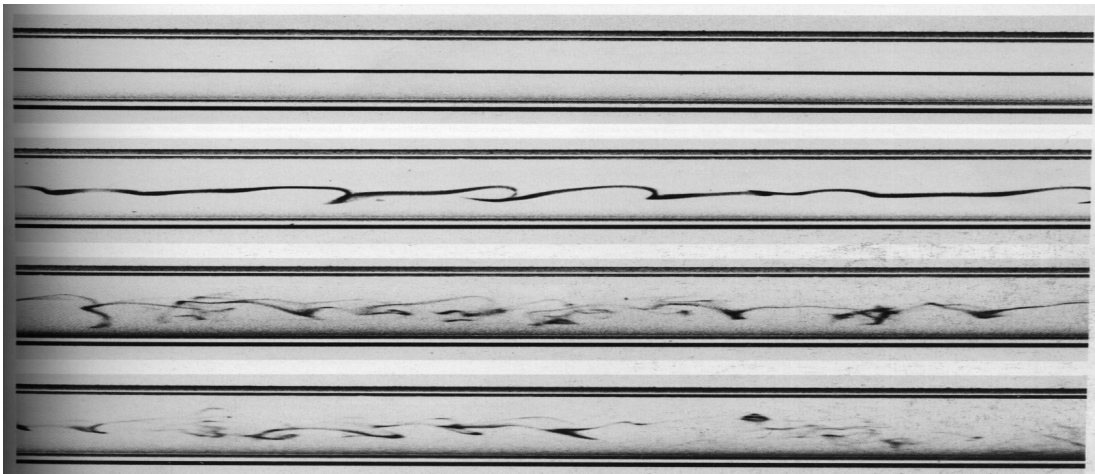
Figure 2.1: Visualization of flow at different Re number in a Reynolds' experiment repetition
