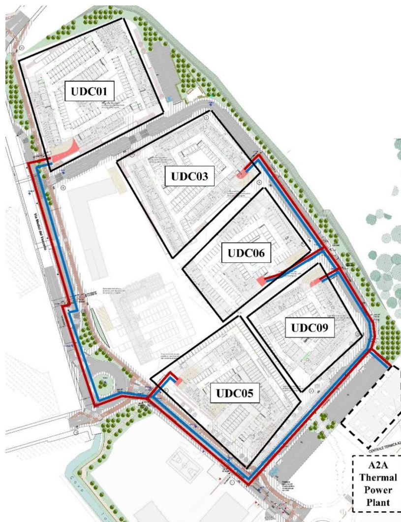
Figure 6.8 Merezzate district heating network
