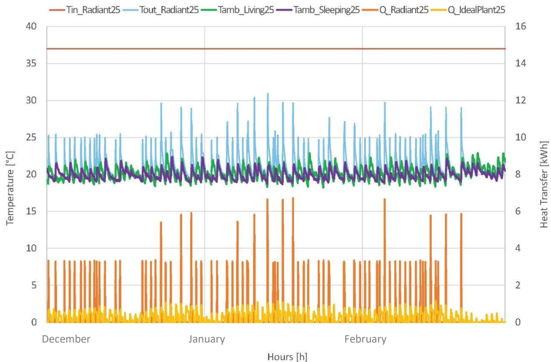
Graph 6.4 Radiant panels data analysed in a short period for flat n°25
