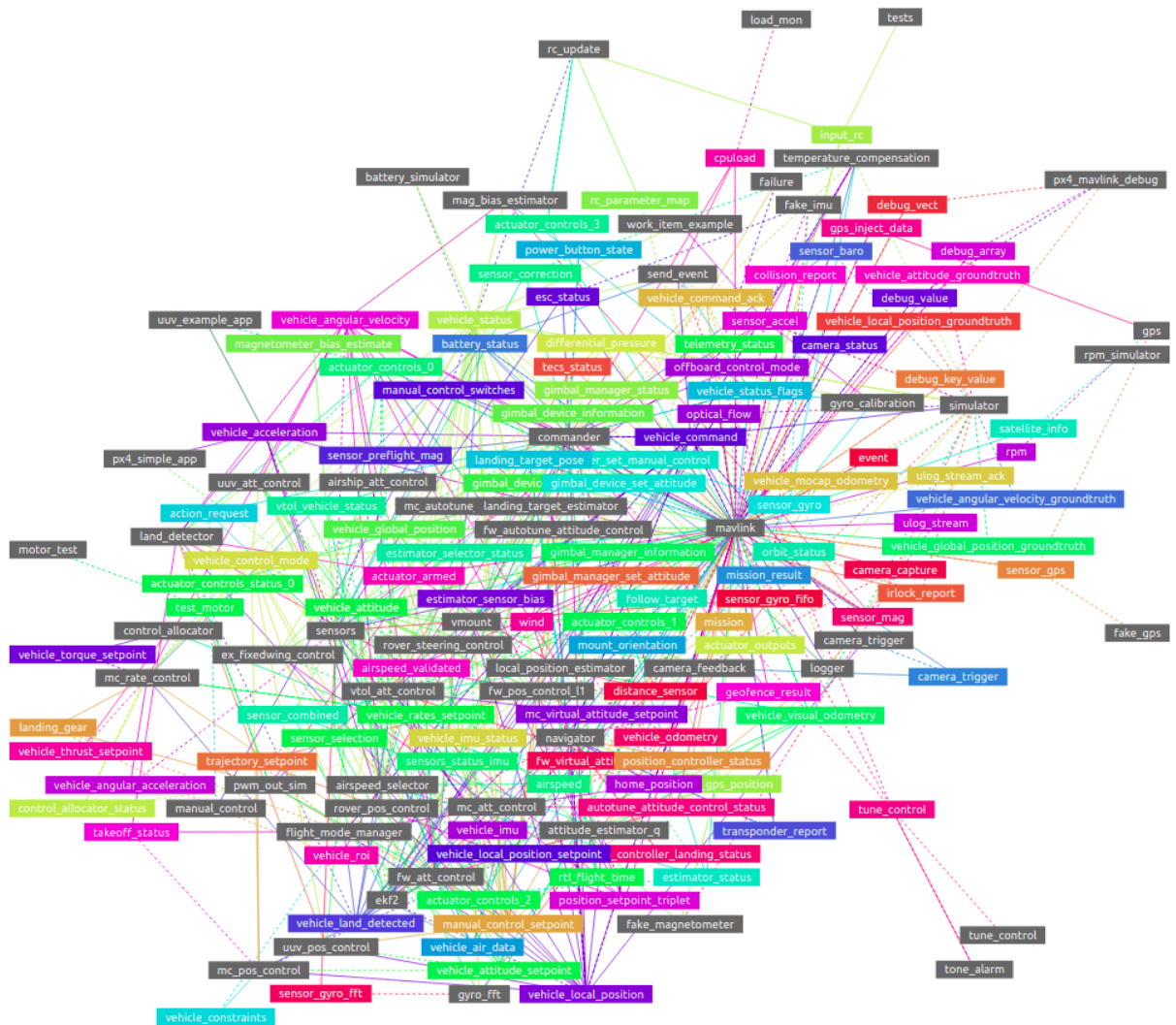
Figure 3.4. uORB graph (old version)
