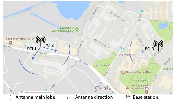
Figure 4.1: Map showing the BS positions and the PCIs in the reference dataset
