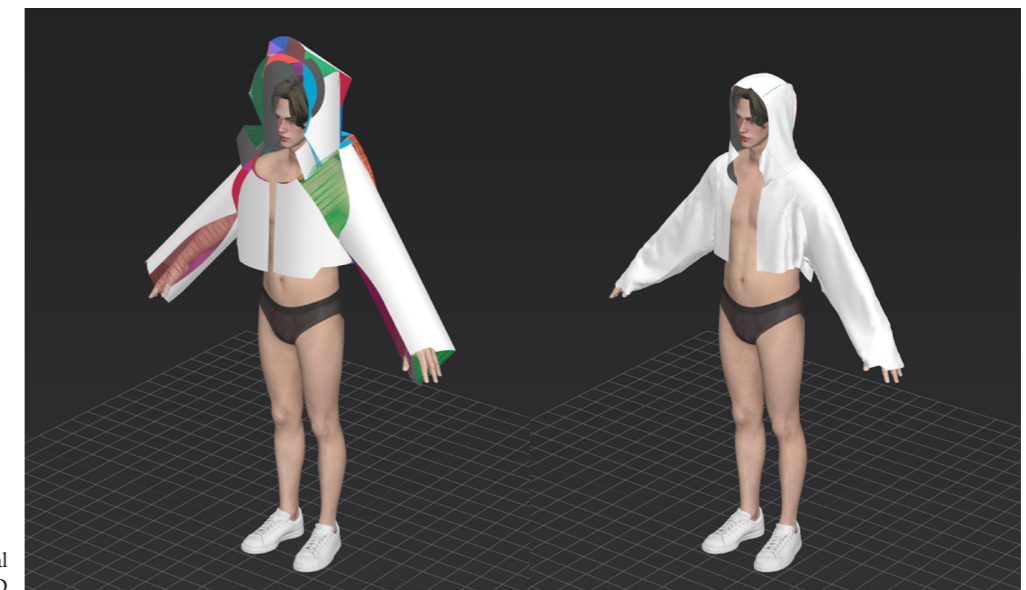
Fig 14. Illustration of virtual sewing in Clo3D
