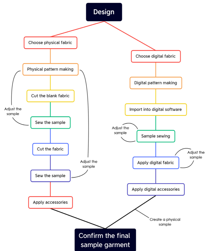
Comparison chart of digital sample garment production and actual sample garment production processes
