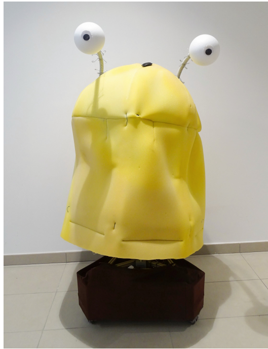
Figure 4.3: The foam under the skin of the robot
