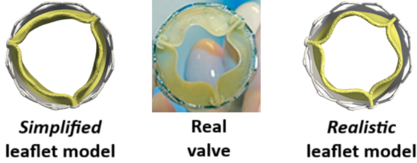
Figure 3.2: Geometrical model for the bio-prosthetic valve's leaflets in open configuration. Left: simplified leaflets model. Center: real valve's leaflets. Right: realistic leaflets model. The image of the real valve is taken from Holoshitz, Kavinsky, Hijazi [117] with written permission by Hijazi.
