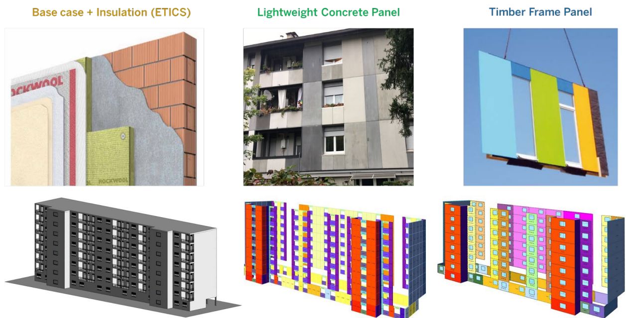
Figure 9: Meta-technological recladding options to compare in the Panelization Design Tool
