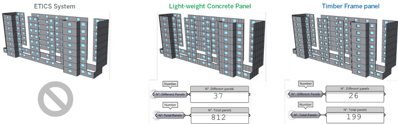
Figure 145: 3D Panels layouts output generating two parameters: the total number of panels and the final estimation of different panels number
