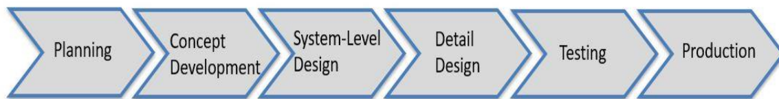
Figure 4: Development Process (Source: Ulrich & Eppinger)
