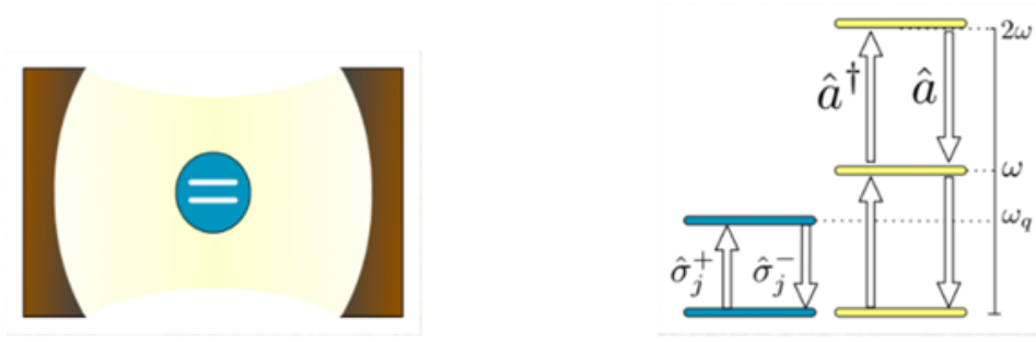
Figure 1.5: Left: scheme of a two-level emitter inside a resonant cavity . Right: energy levels scheme for linear light-matter coupling.
