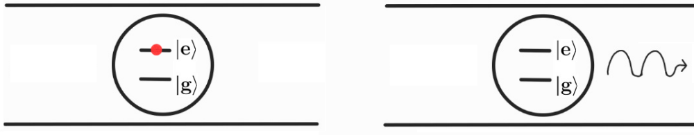
Figure 2.2: Left: at time t_0 the qubit is in the excited state |e\rangle . Right: after a certain amount of time the qubit spontaneously emits a photon and relaxes in the ground state |g\rangle . In principle the emission could be in the right or in the left direction with a certain probability.
