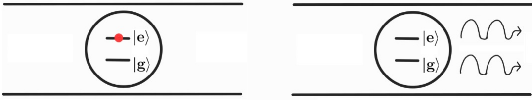
Figure 3.2: Left: at time t_0 the qubit is in the excited state |e\rangle . Right: after a certain amount of time the qubit spontaneously emits two photons and relaxes in the ground state |g\rangle . In principle the emitted photons could propagate in different directions with respect to that showed here with a certain probability.
