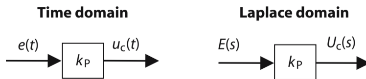
Figure 2-11: Block diagrams of the proportional control term [24]
