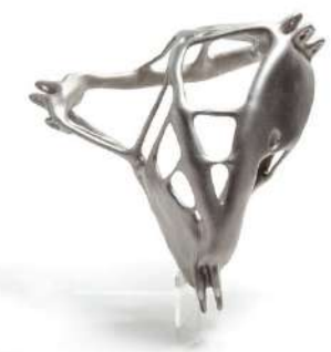
Figure 105-3.3 3D Printed Stainless Steel Node, Prototyped (Manuel Muehlbauer, 2017)
