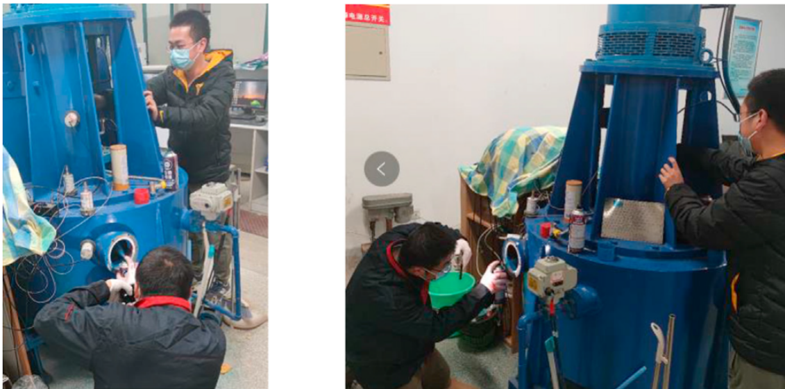
Figure 1.6: An example of experimental setup for testing turbine erosion (picture from Ge et al. [5]).
