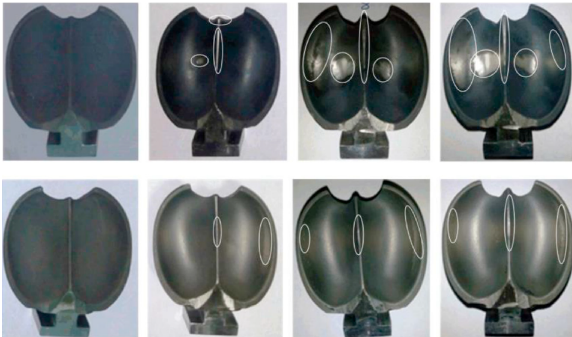
Figure 1.2: Process of erosion of a Pelton turbine blade. Different jet velocities, silt sizes and concentrations are considered in the two cases. The blade is shown at different time instants (picture from Ge et al. [5]).
