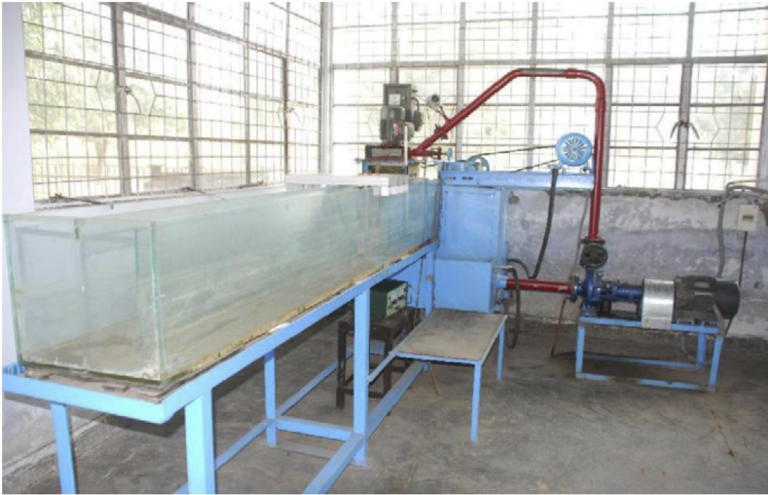
Figure 1.7: Another example of experimental setup for testing turbine erosion (picture from Padhy [13]).
