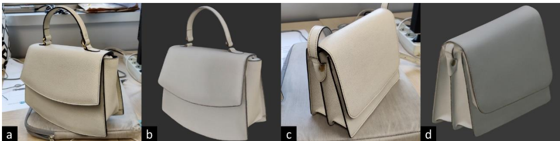
Figure 7.1 - Physical prototypes (a & c) and their corresponding reconstructed textured 3D model (b & d)
