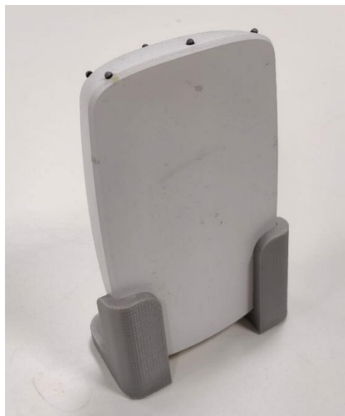
Figure 2.4 - Physical prototype painted with a white matte finish
