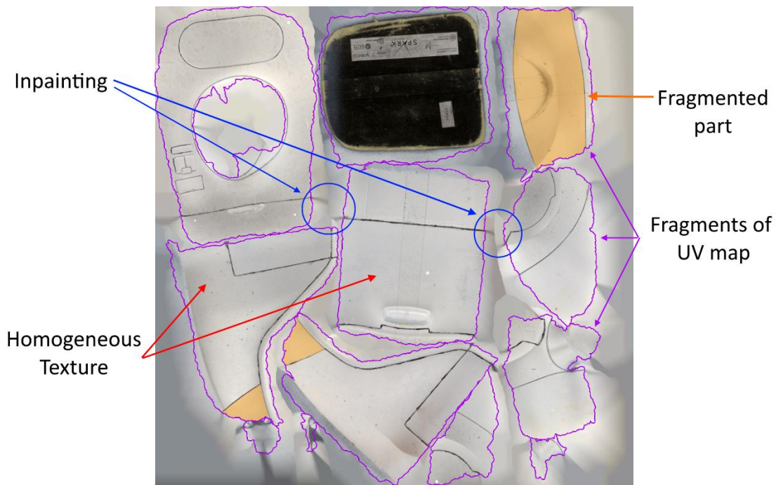
Figure 2.15 - Characteristics of surface reconstructed textures of mixed prototypes
