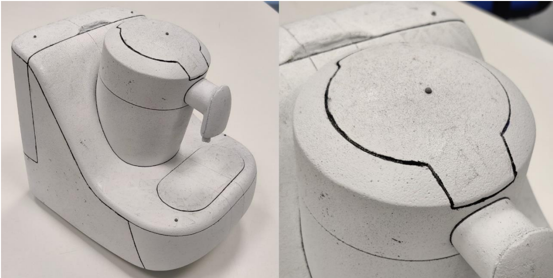
Figure 6.8 – Prepared coffee machine physical prototype (left) with close-up of added features (right)
