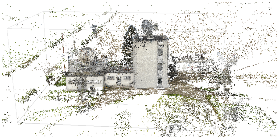
Figure 40 - Sparse point cloud for medium accuracy
