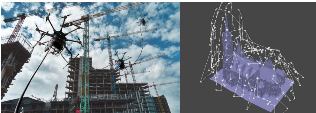
Figure 5 - Cable connected drones and their movement (Source: Bolognini, Michele - PhD Thesis)
