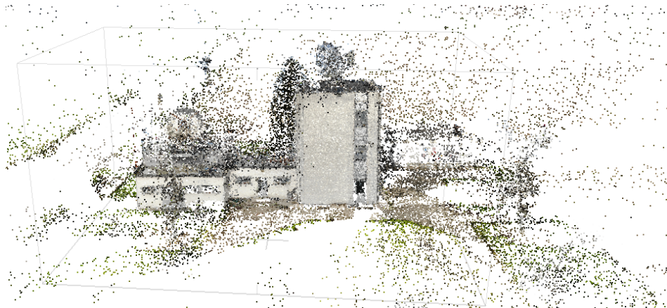
Figure 40 - Sparse point cloud for medium accuracy
