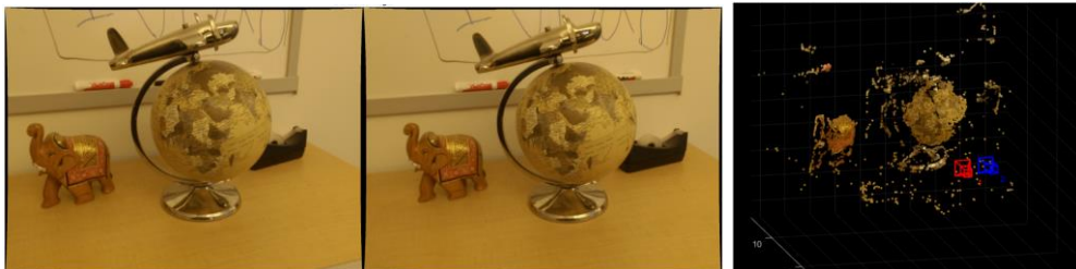
Figure 22 - Example of 3D reconstruction by Matlab (Source: Matlab – Structure from Motion from multiple views - https://it.mathworks.com/help/vision/ug/structure-from-motion-from-two-views.html )
