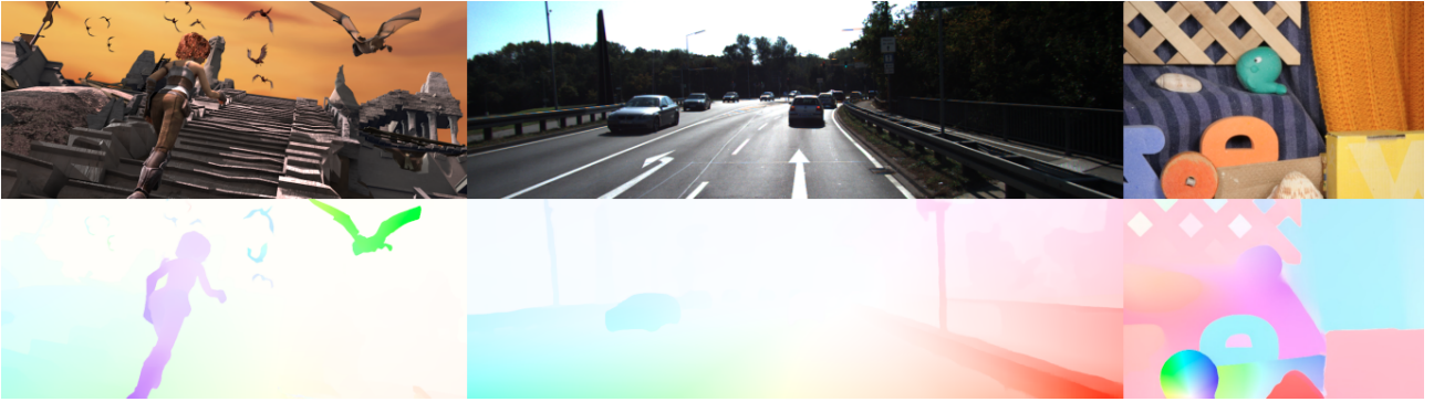
Figure 2: Optical flow predictions from SEA-RAFT [54] on Sintel [3] (test), KITTI2015 [12] (test), and Middlebury [1] (train). Top row: input frames. Bottom row: predicted flow visualized using the standard HSV color encoding, where color encodes direction and brightness encodes magnitude. Figure taken from [54].
