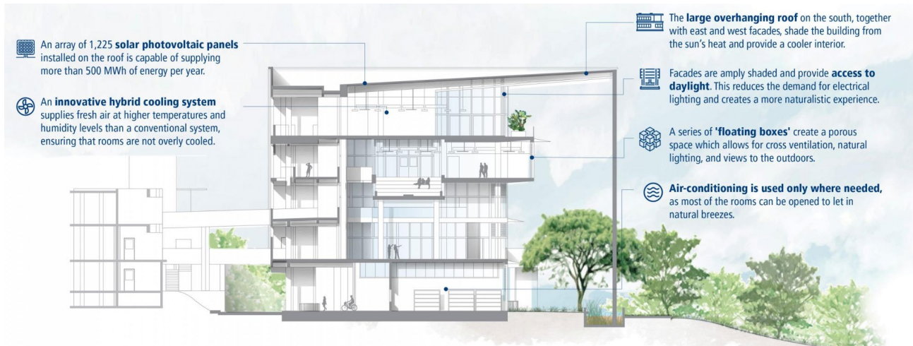
Figure 67. Sectional diagram illustrating SDE4's integrated passive and active environmental strategies. National University of Singapore, 2019)
