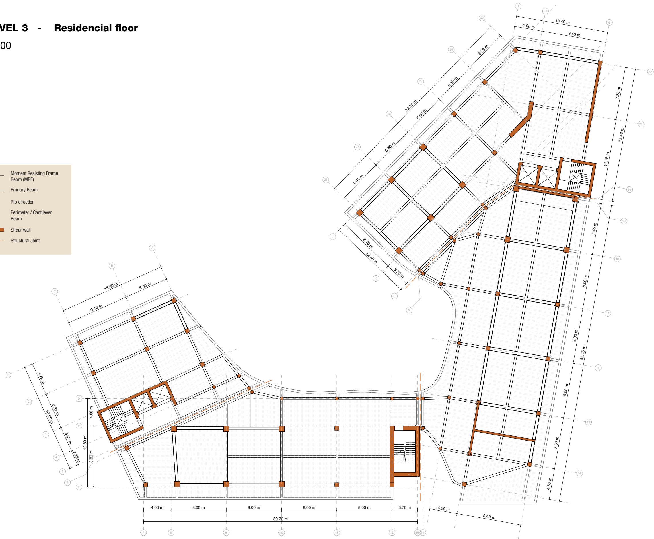
Figure 112. Residential floor typical structural plan. (Author, 2026).
