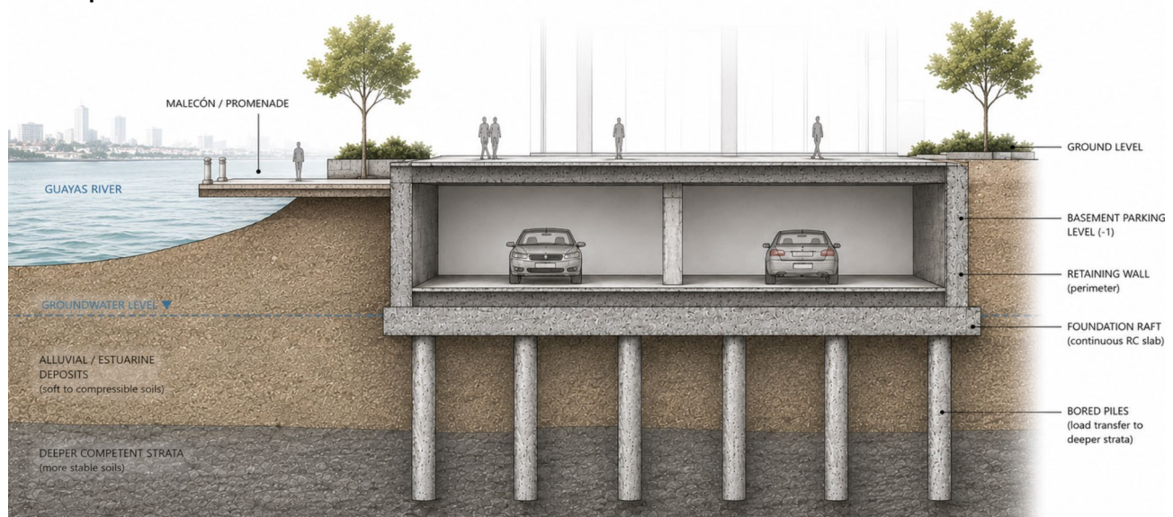
Figure 113. Conceptual foundation strategy illustrating the proposed piled raft system
