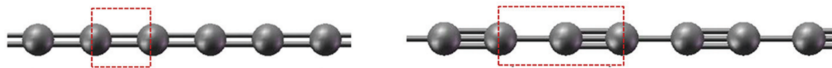
Figure 1.2: Sketch of a cumulene on the left and on the right of a polyynes. Adapted from [5].
