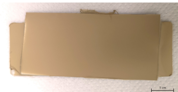
Figure 5.3: PVA nanofibers with concentrated AgNPs and PLAL water polyynes mixture electrospun for 1h.
