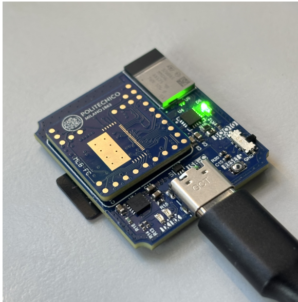
Figure 3.20: Green LED: Standalone operational mode.
