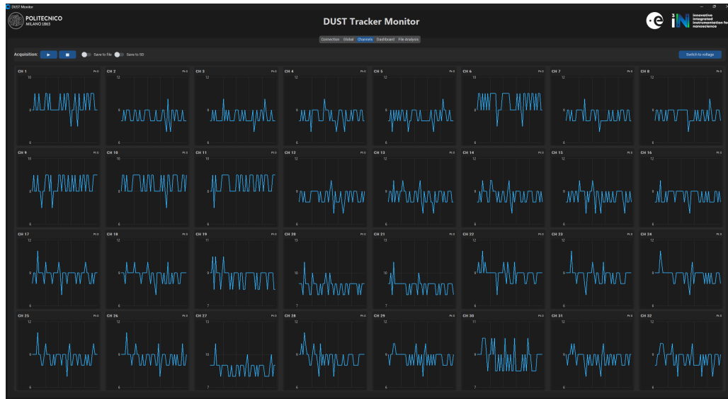
Figure 4.8: Visualization of the initial floating state of the electrodes before the analog front-end biasing is fully stabilized.
