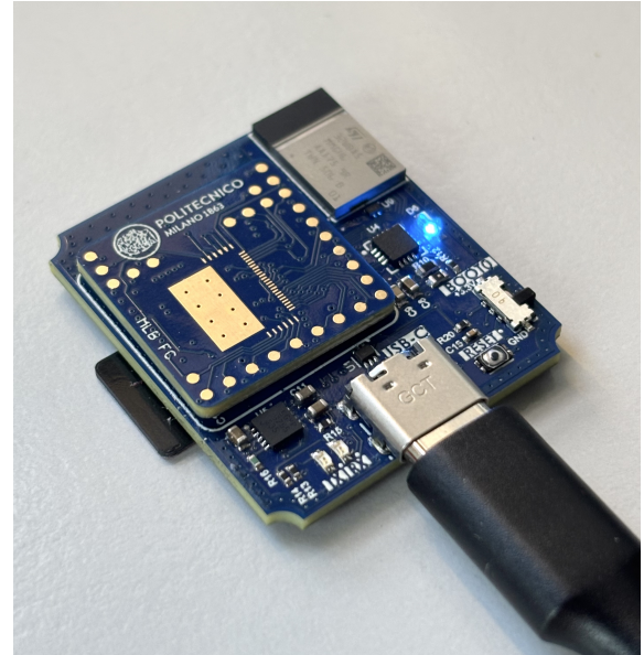
Figure 3.21: Blue LED: Active and stable BLE connection.
