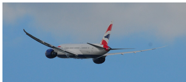
Figure 1: Boeing 787-8 Dreamliner, whose wings are flexed upward by pressure forces. Images taken from [6]
