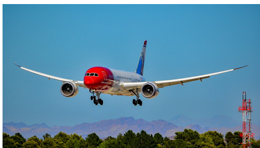
Figure 1: Boeing 787-8 Dreamliner, whose wings are flexed upward by pressure forces. Images taken from [6]
