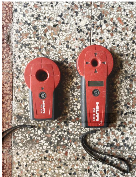
Figure 30 - Instrument for the wall thickness measurement
