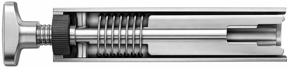
fig. 48 Render section of the height adjustment mechanism
