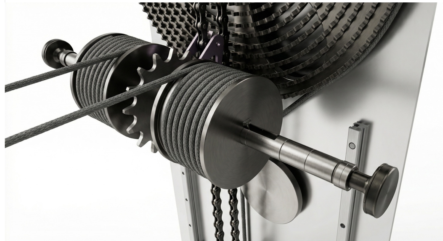
fig. 47 The drums and vertical adjustment system
