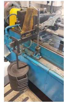
Figure 5.1: The Calibration Setup Installed on the FZG Hypoid Test Rig
